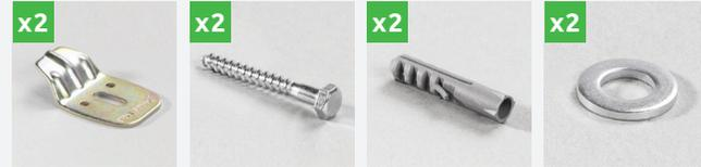
The kit includes two main vertical brackets designed to clamp onto the basins back strap and fit to the wall. These brackets can be adjusted to the correct height/position required. The plugs have a two-way expansion mechanism that provides a strong anchorage in solid base materials. The screws can also be used to install into timber.
