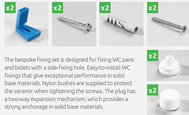
The bespoke fixing set is designed for fixing WC pans and bidets with a side-fixing hole. Easy-to-install WC fixings that give exceptional performance in solid base materials. Nylon bushes are supplied to protect the ceramic when tightening the screws. The plug has a two-way expansion mechanism, which provides a strong anchorage in solid base materials.
