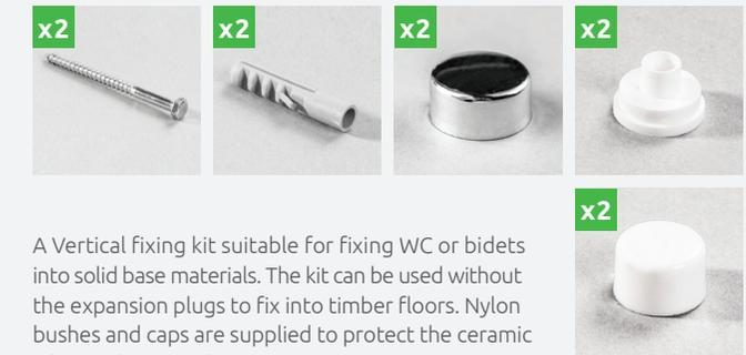
A Vertical fixing kit suitable for fixing WC or bidets into solid base materials. The kit can be used without the expansion plugs to fix into timber floors. Nylon bushes and caps are supplied to protect the ceramic when tightening the screws.
