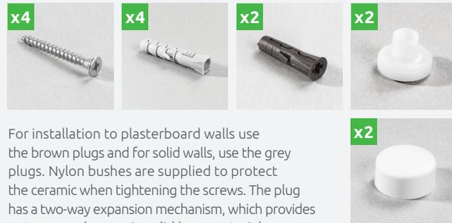
For installation to plasterboard walls use the brown plugs and for solid walls, use the grey plugs. Nylon bushes are supplied to protect the ceramic when tightening the screws. The plug has a two-way expansion mechanism, which provides a strong anchorage in solid base materials.
