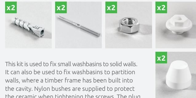
This kit is used to fix small washbasins to solid walls. It can also be used to fix washbasins to partition walls, where a timber frame has been built into the cavity. Nylon bushes are supplied to protect the ceramic when tightening the screws. The plug has a two-way expansion mechanism, which provides a strong anchorage in solid base materials.
